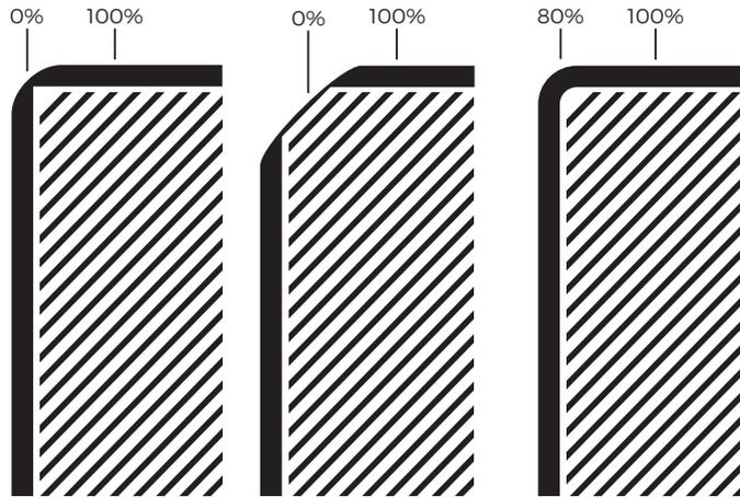
The illustration shows how the coating film build is affected by a sharp edge detail creating a chamfer reduces the acute angle of the sharp edge, but introduces a second edge. The coating film created over a 3 mm radius edge is 80%. Linking this with the minimum coating film thickness, an applied film of 120 µm on the face of the joinery would achieve a coating film of approximately 95 µm.
