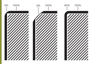
The illustration shows how the coating film build is affected by a sharp edge detail creating a chamfer reduces the acute angle of the sharp edge, but introduces a second edge. The coating film created over a 3 mm radius edge is 80%. Linking this with the minimum coating film thickness, an applied film of 120  $\mu$ m on the face of the joinery would achieve a coating film of approximately 95  $\mu$ m.
